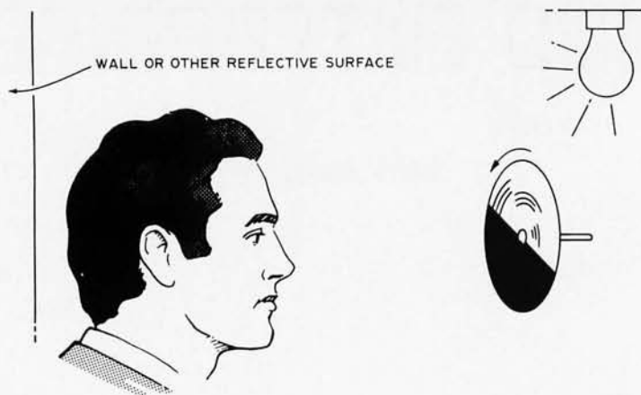
Figure 2: A suggested geometry of illumination for viewing the Benham disk.
